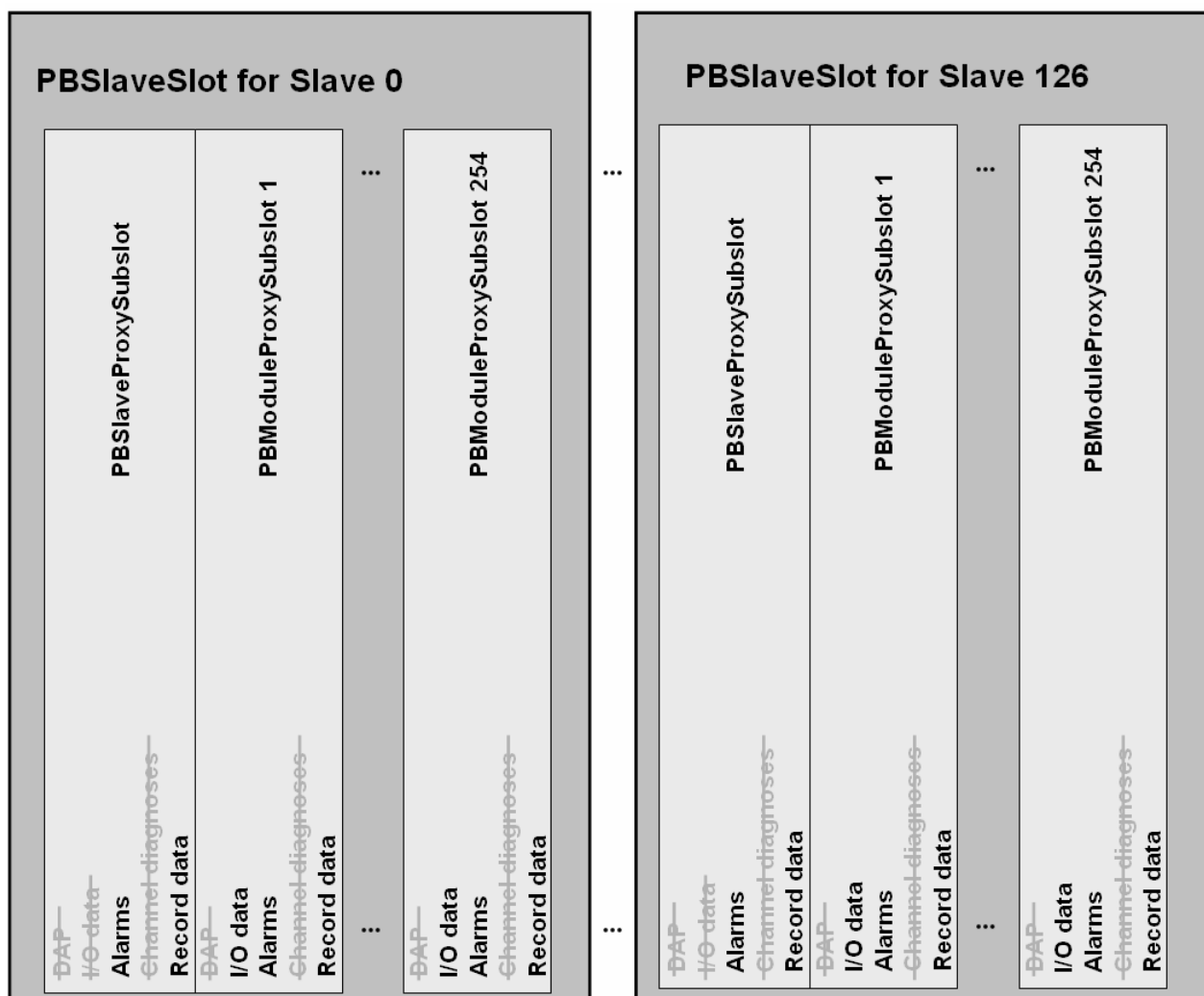
Figure 12: Modelling of the submodules of PROFIBUS slaves at the 1 st Master System
