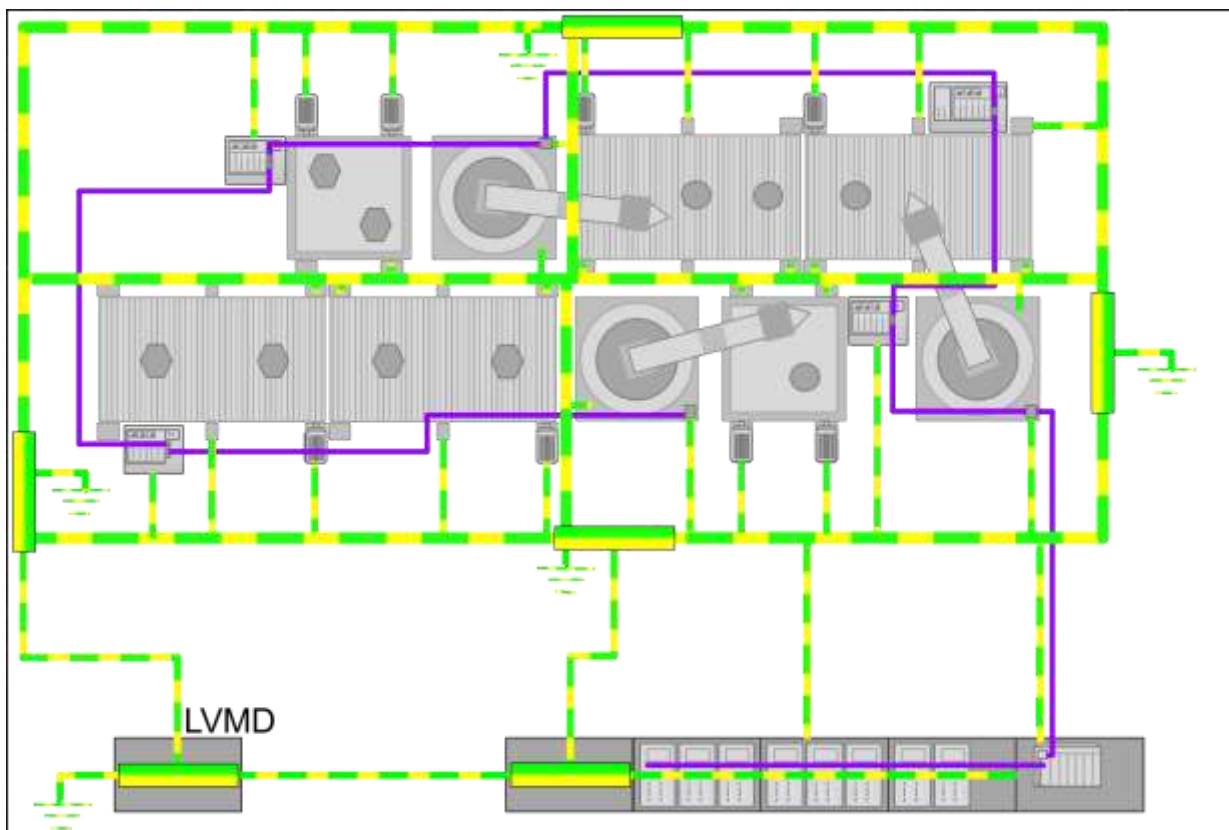
Figure 4.30: Meshed equipotential bonding
