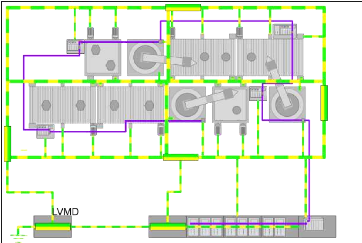
Figure 4.32: Stubs of the meshed equipotential bonding system
