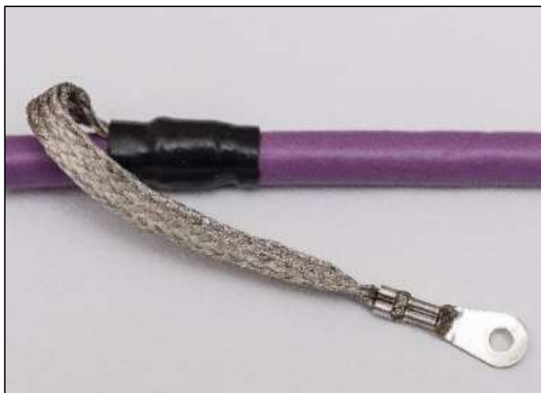
Figure 4.42: Additional connection of the cable shield [NIE2017]
